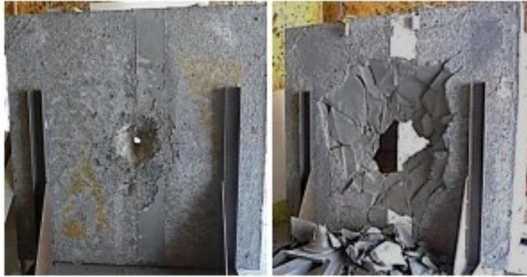
Figure 1.2 Impact Experiments of Concrete with (left) and without (right) fiber reinforcement (Pontiroli, 2019)
