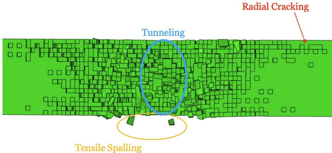
Figure 5.2 Aspects of the ballistic impact seen throughout the target of a ballistic impact simulation with an initial velocity of  $1000\text{ms}^{-1}$  and target thickness of 1in.
